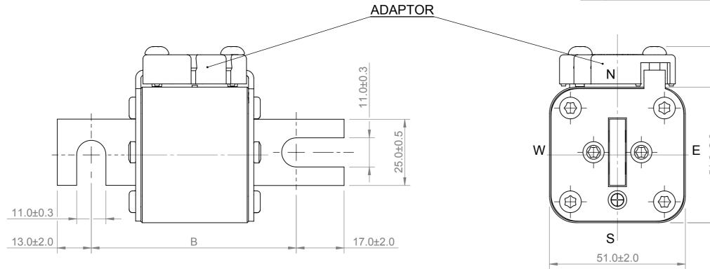
The normal position of the indicator is as shown position N.
