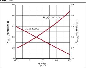
**FIGURE 2-11:**  $V_{GS(th)}$  and  $R_{DS}$  Variation with Temperature.
