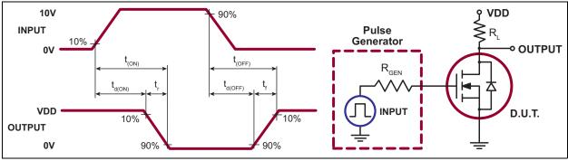
FIGURE 4-1: Switching Waveforms and Test Circuit.
