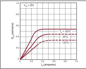
FIGURE 2-2: Transconductance vs. Drain Current.
