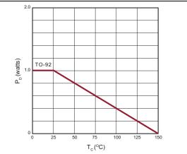
FIGURE 2-5:Power Dissipation vs. CaseTemperature.
