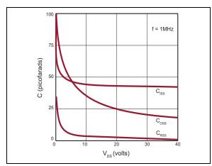
FIGURE 2-9: Capacitance vs. Drain-to-Source Voltage.
