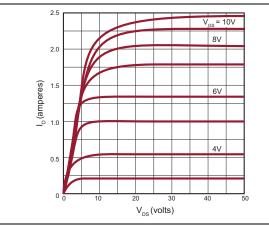
FIGURE 2-1: Output Characteristics.
