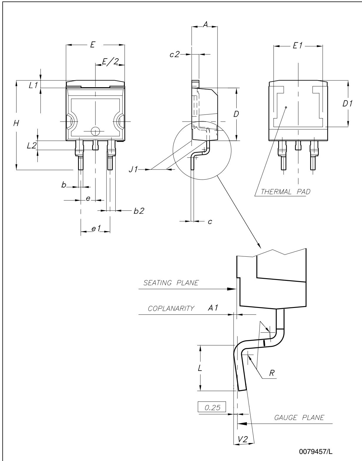
**Figure 13.** Drawing dimension D<sup>2</sup>PAK (type WOOSEOK-Subcon.)
