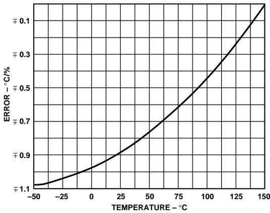
Figure 4. Setpoint Error Due to  $R_{SET}$  Tolerance
