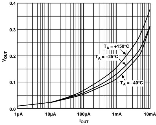
Figure 9.  $V_{OUT}$  vs.  $I_{OUT}$  ( $V_{OUT} = LOW$ )
