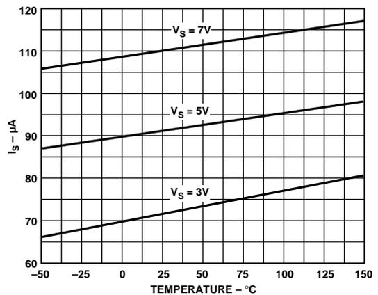
Figure 8. Supply Current vs. Temperature ( $V_{OUT} = LOW$ )
