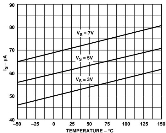
Figure 5. Supply Current vs. Temperature ( $V_{OUT} = HIGH$ )
