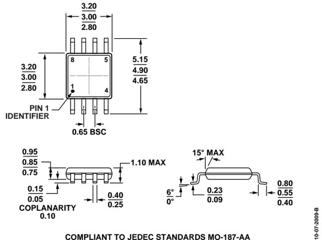
Figure 36. 8-Lead Mini Small Outline Package [MSOP] (RM-8)
