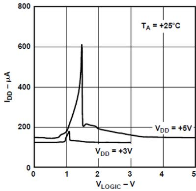
Figure 17. Supply Current vs. Logic Input Voltage
