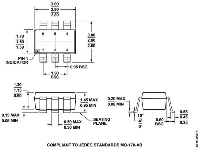
Figure 35. 6-Lead Small Outline Transistor Package [SOT-23] (RJ-6)
