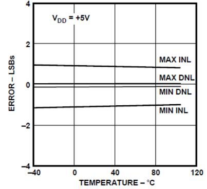
Figure 8. INL Error and DNL Error vs. Temperature
