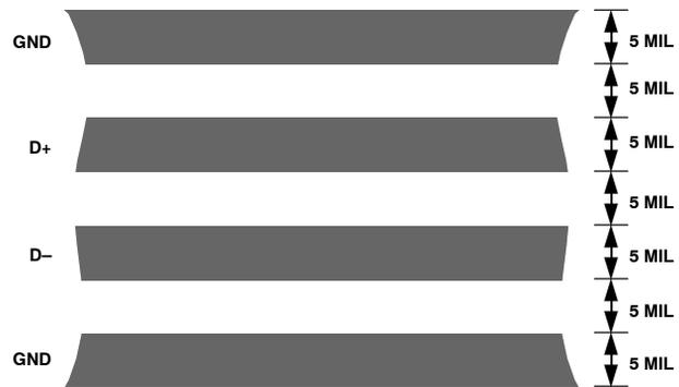
**Figure 23. Typical Arrangement of Signal Tracks**
