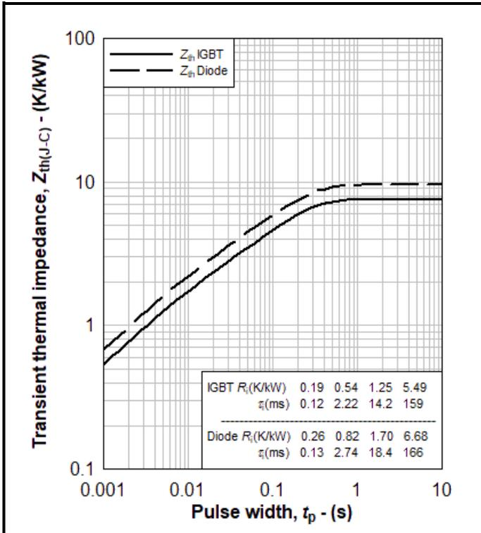
Fig. 13 Transient thermal impedance,  $Z_{th(J-C)} = f(t)$
