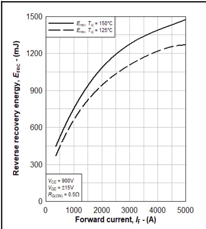
Fig. 9 Typical FRD  $E_{rec}$ ,  $E_{rec} = f(I_F)$
