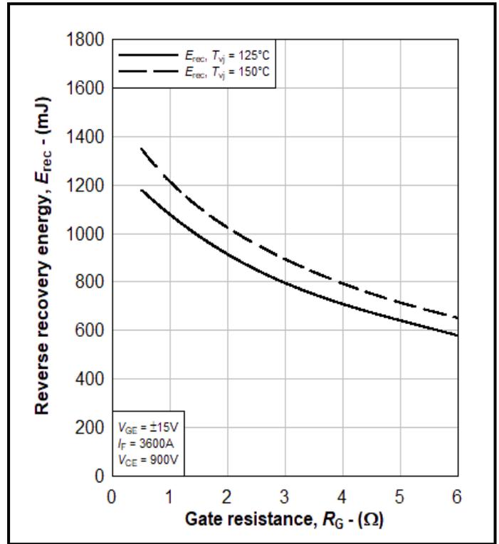
Fig. 8 Typical FRD  $E_{rec}$ ,  $E_{rec} = f(R_G)$
