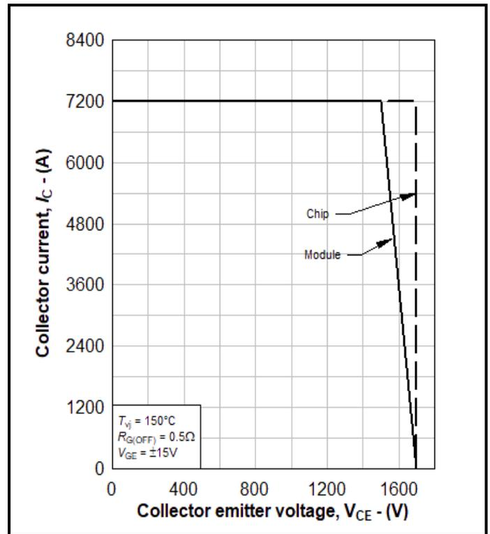
Fig. 12 Reverse bias safe operating area of IGBT,
