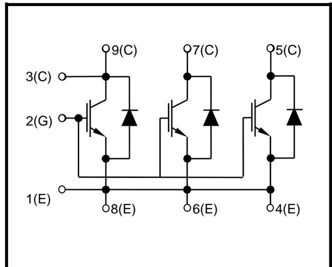
**Fig. 1 Circuit configuration**
