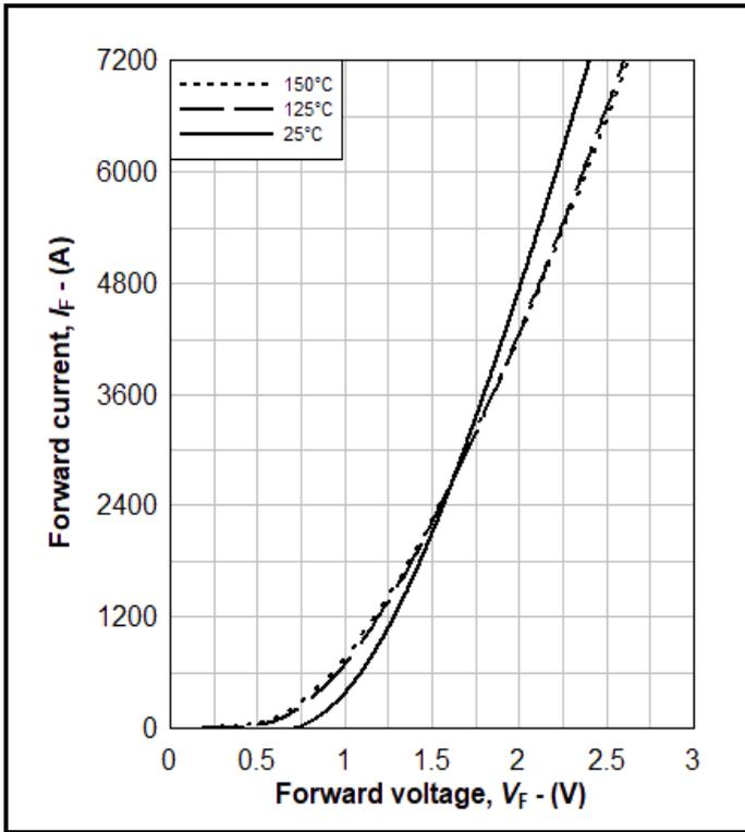
Fig. 7 Typical FRD output characteristics,  $I_F = f(V_F)$
