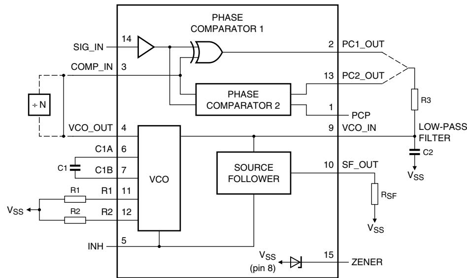
**Fig 1.** Functional diagram
