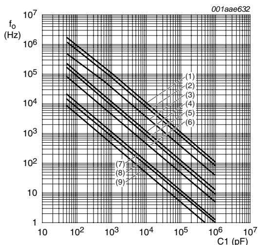
$T_{\text{amb}} = 25^\circ\text{C}$ ; VCO\_IN at  $0.5V_{DD}$ ; INH\_IN at  $V_{SS}$ ;  $R2 = \infty$ .
