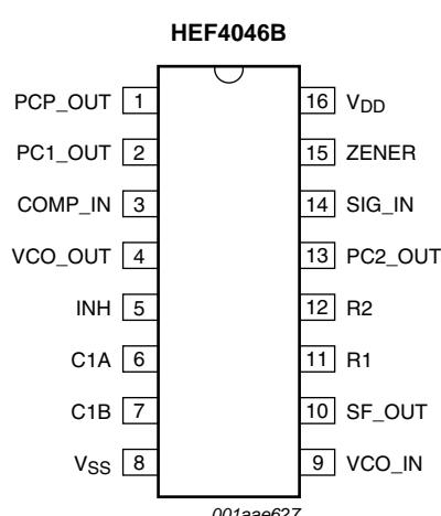
**Fig 2.** Pin configuration
