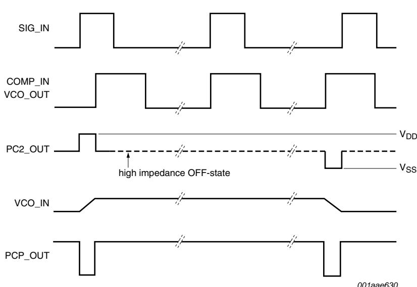
**Fig 5. Typical waveforms for phase-locked loop with a locked phase comparator 2**
