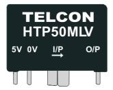
The HTP50MLV is a closed loop Hall Effect Current Transformer suitable for measuring currents up to 50A and operating from a single +5V power supply. The product provides an output voltage, proportional to the current in the galvanically isolated primary conductor, centred on 2.5V. This enables measurement of bi-polar currents.
