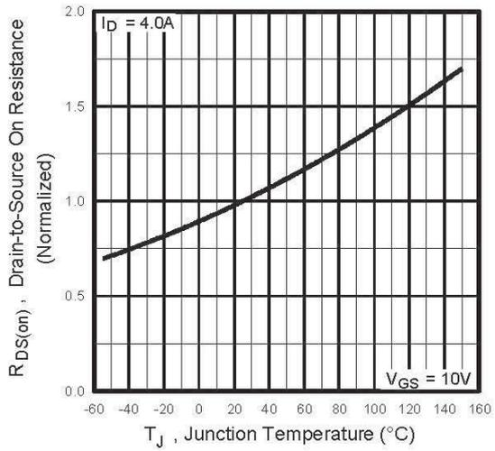
**Fig 4.** Normalized On-Resistance
