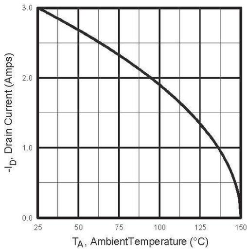
Fig 20. Max. Drain Current Vs. Ambient Temp.
