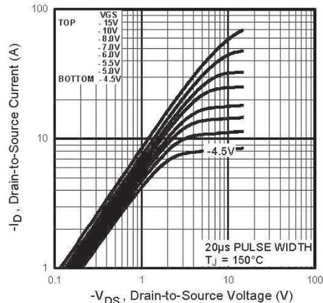
Fig 13. Typical Output Characteristics,  $T_J = 150^\circ\text{C}$
