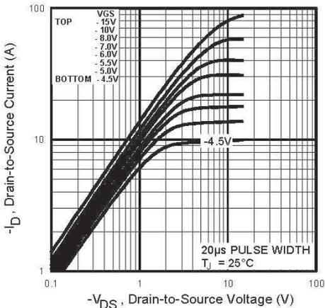
Fig 12. Typical Output Characteristics,  $T_J = 25^\circ\text{C}$
