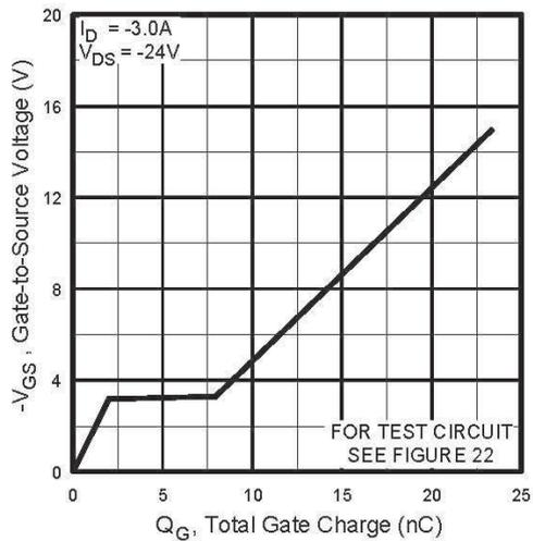
Fig 17. Typical Gate Charge Vs. Gate-to-Source Voltage
