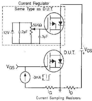
Fig 22b. Gate Charge Test Circuit
