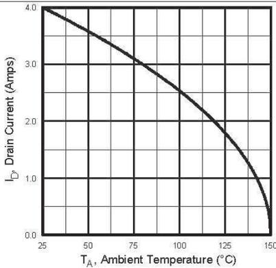
Fig 9. Max. Drain Current Vs. Ambient Temp.
