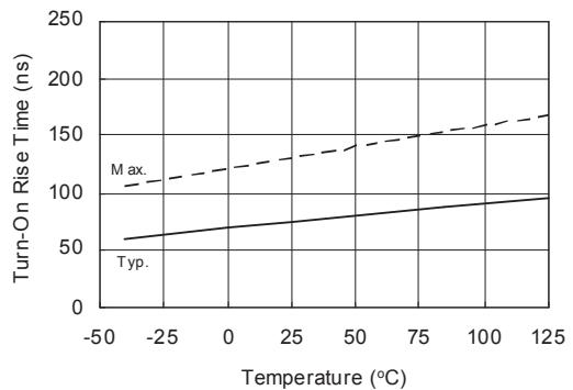
**Figure 10A. Turn-On Rise Time vs. Temperature**
