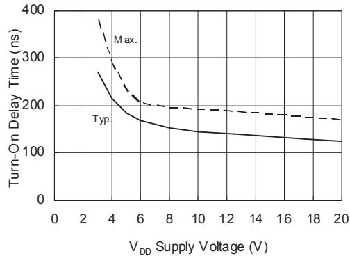
Figure 7C. Turn-On Propagation Delay Time vs.  $\text{V}_{\text{DD}}$  Supply Voltage
