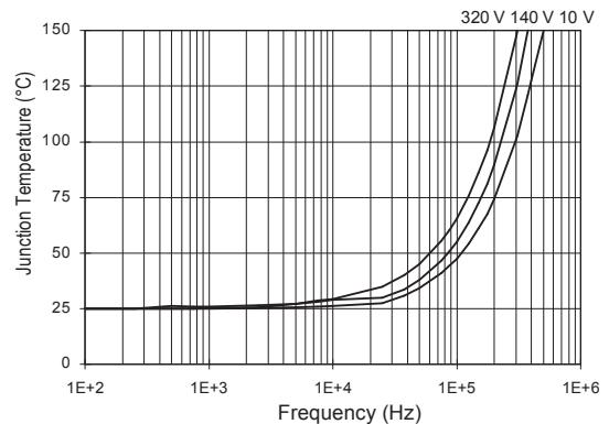
**Figure 35. IRS2112S  $T_J$  vs. Frequency (IRFPE50)**
