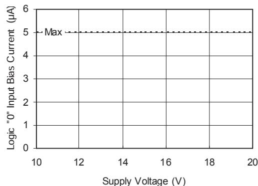
Figure 21B. Logic "0" Input Bias Current vs. Voltage
