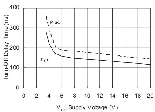
Figure 8C. Turn-Off Propagation Delay Time vs.  $\text{V}_{\text{DD}}$  Supply Voltage
