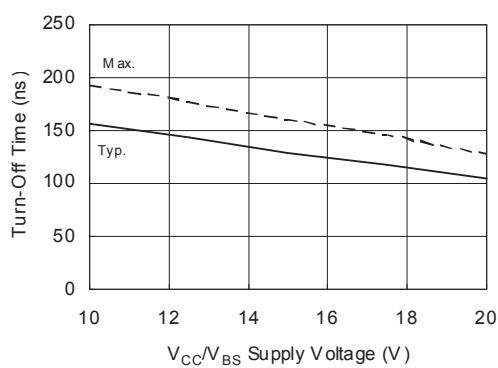
Figure 8B. Turn-Off Propagation Delay Time vs.  $\text{V}_{\text{CC}}/\text{V}_{\text{BS}}$  Supply Voltage
