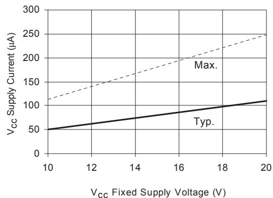
Figure 18B. V<sub>CC</sub> Supply Current vs. Voltage
