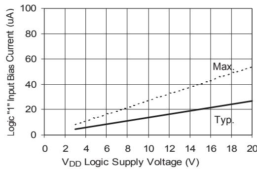
Figure 20B. Logic "1" Input Current vs. V<sub>DD</sub> Voltage
