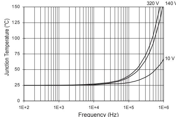
**Figure 33. IRS2112S  $T_J$  vs. Frequency (IRFBC30)**
