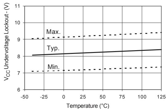
**Figure 25.**  $V_{CC}$  Undervoltage Lockout (-) vs. Temperature
