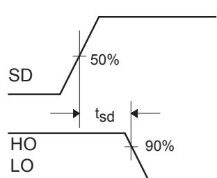
**Figure 5. Shutdown Waveform Definitions**
