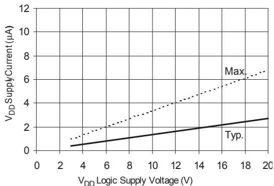
Figure 19B. V<sub>DD</sub> Supply Current vs. V<sub>DD</sub> Voltage
