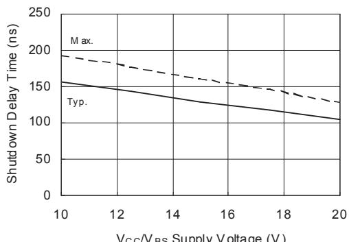
**Figure 9B. Shutdown Delay Time vs. V<sub>CC/V<sub>BS</sub></sub> Supply Voltage**
