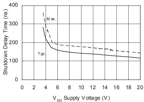
**Figure 9C. Shutdown Time vs. V<sub>DD</sub> Supply Voltage**
