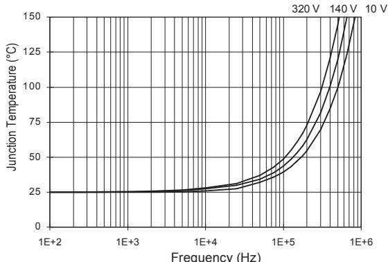
**Figure 31. IRS2112  $T_J$  vs. Frequency (IRFPE50)**
