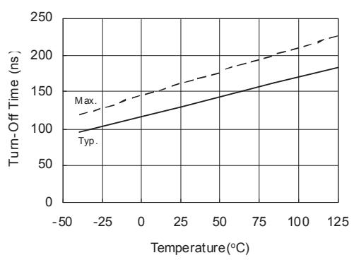
Figure 8A. Turn-Off Propagation Delay Time vs. Temperature
