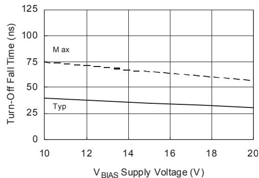
Figure 11B. Turn-Off Fall Time vs. Supply Voltage
