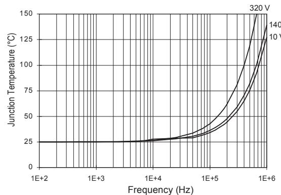
**Figure 34. IRS2112S  $T_J$  vs. Frequency (IRFBC40)**
