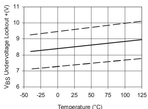
Figure 22. V<sub>BS</sub> Undervoltage Lockout (+) vs. Temperature
