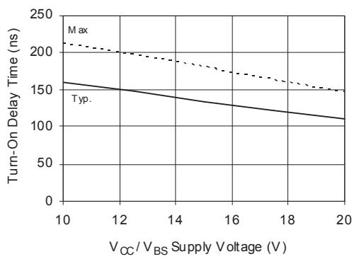
Figure 7B. Turn-On Propagation Delay Time vs.  $\text{V}_{\text{CC}}/\text{V}_{\text{BS}}$  Supply Voltage
