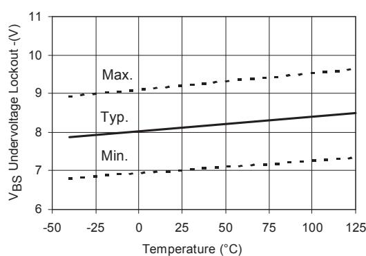
Figure 23. V<sub>BS</sub> Undervoltage (-) vs. Temperature
