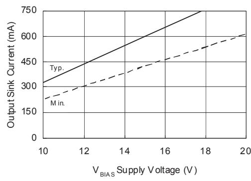
**Figure 27B.** Output Sink Current vs. Supply Voltage
