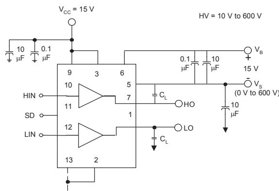
**Figure 3. Switching Time Test Circuit**
