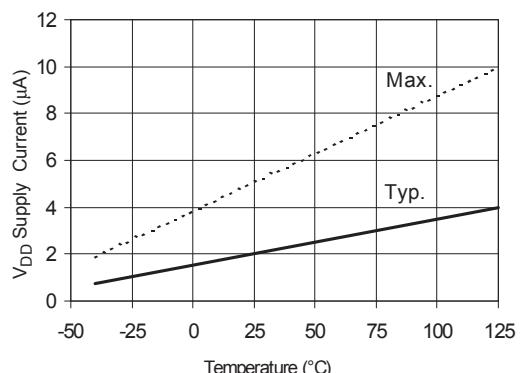
Figure 19A. V<sub>DD</sub> Supply Current vs. Temperature
