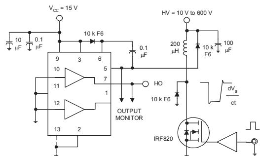
**Figure 2. Floating Supply Voltage Transient Test Circuit**
