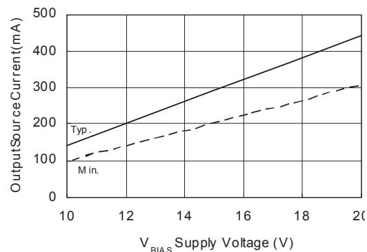
**Figure 26B.** Output Source Current vs. Supply Voltage
