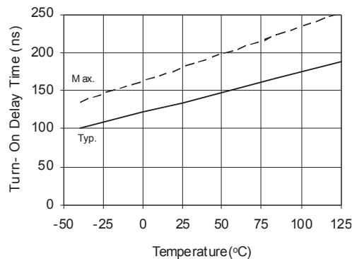
Figure 7A. Turn-On Propagation Delay Time vs. Temperature
