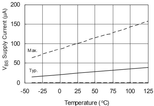
**Figure 16A.  $V_{BS}$  Supply Current vs. Temperature**
