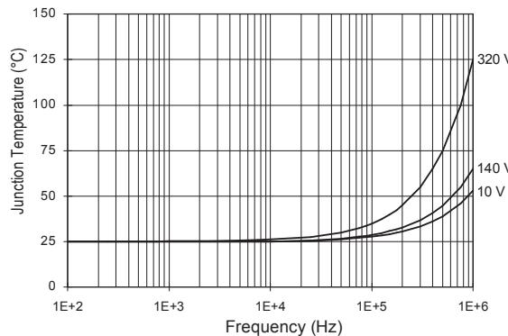
**Figure 28. IRS2112  $T_J$  vs. Frequency (IRFBC20)**
