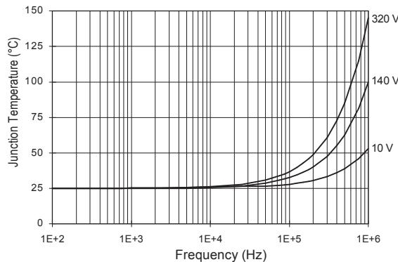
**Figure 29. IRS2112  $T_J$  vs. Frequency (IRFBC30)**
