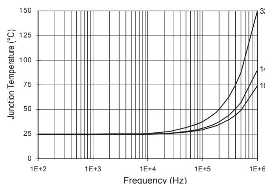
**Figure 32. IRS2112S  $T_J$  vs. Frequency (IRFBC20)**
