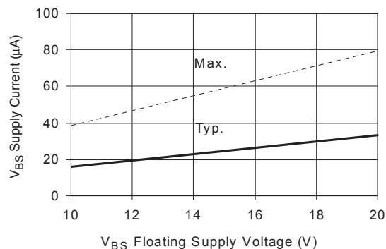
Figure 17B. V<sub>BS</sub> Supply Current vs. Voltage
