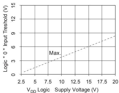
Figure 13B. Logic "0" Input Threshold vs. Voltage
