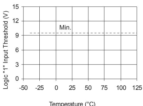
Figure 12A. Logic "1" Input Threshold vs. Temperature
