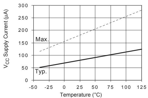
Figure 18A. V<sub>CC</sub> Supply Current vs. Temperature
