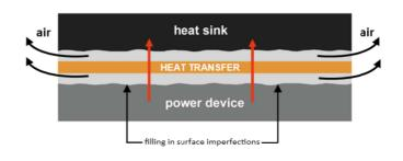
Note: during initial phase-change, it is recommended to re-check your torque settings if device utilizes a screw mounting system. Applying additional torque during initial phase change will thin the material bond line slightly leading to improved thermal performance.
