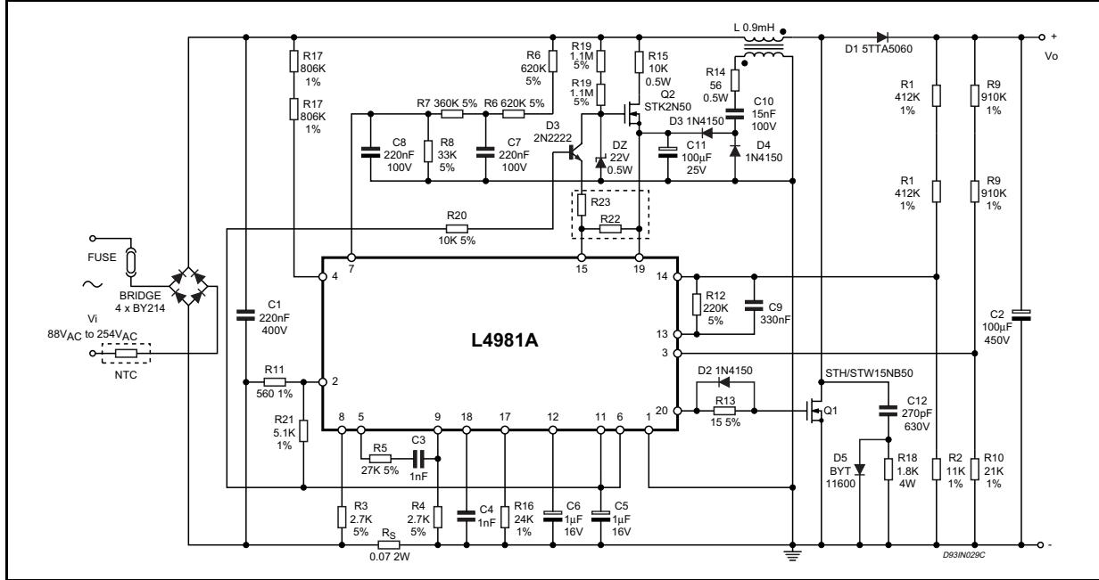
$f_{SW} = 80\text{kHz}$ ;  $P_O = 200\text{W}$ ;  $V_{OUT} = 400\text{V}$ ;  $I_{rms\ max} = 2.53\text{A}$ ;  $V_{OVP} = 442\text{V}$ ;  $I_{PK\ max} = 6.2\text{A}$
