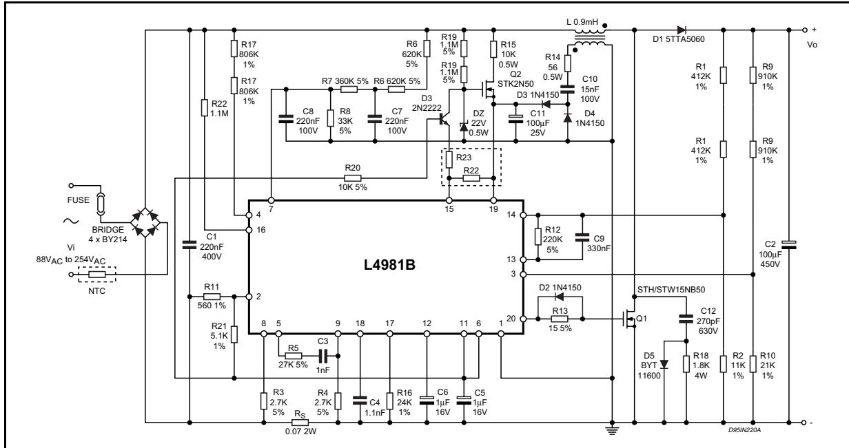
$f_{SW} = 80 \text{ to } 92\text{kHz}$ ;  $P_O = 200\text{W}$ ;  $V_{OUT} = 400\text{V}$ ;  $I_{rms\ max} = 2.53\text{A}$ ;  $V_{OVP} = 442\text{V}$ ;  $I_{PK\ max} = 6.2\text{A}$
