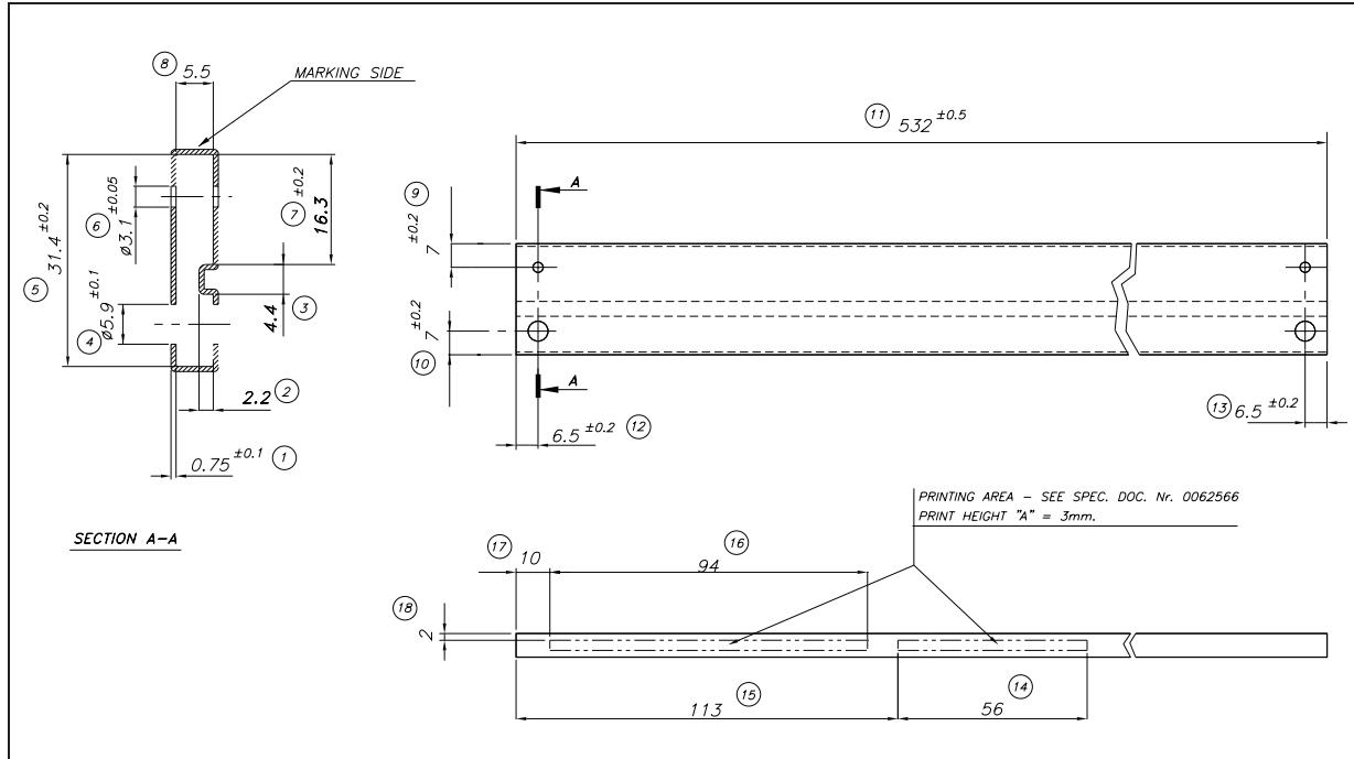
**Figure 32.** Drawing dimension tube for TO-220 Single Gauge (mm.)
