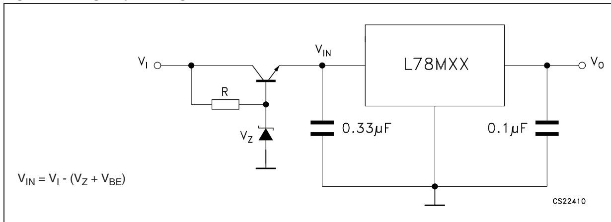
**Figure 26.** Reducing power dissipation with dropping resistor
