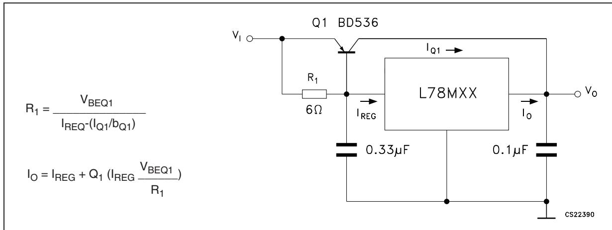
**Figure 23.** High output current with short circuit protection
