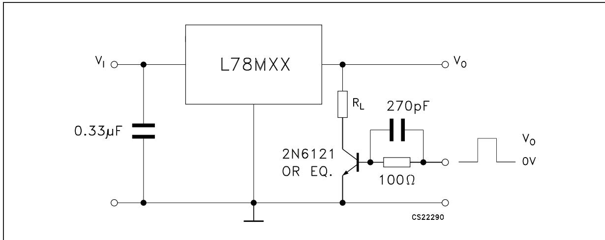
**Figure 7.** Ripple rejection
