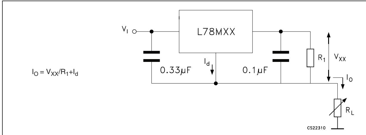
**Figure 19. Circuit for increasing output voltage**
