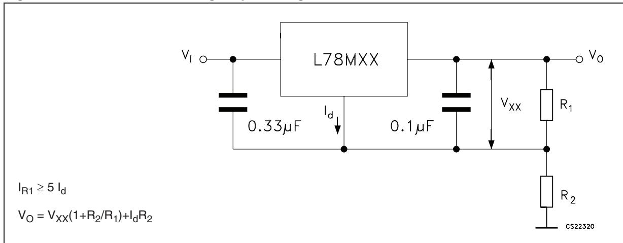
**Figure 20. Adjustable output regulator (7 to 30 V)**
