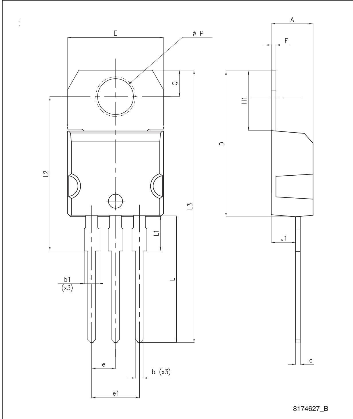
**Figure 31.** Drawing dimension tube for TO-220 Dual Gauge (mm.)
