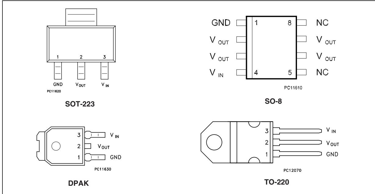
Note: The TAB is connected to the V<sub>OUT</sub>.
