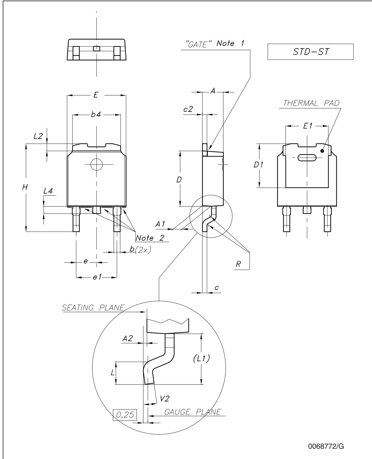
Note: 1 Maximum resin gate protrusion: 0.5 mm.
