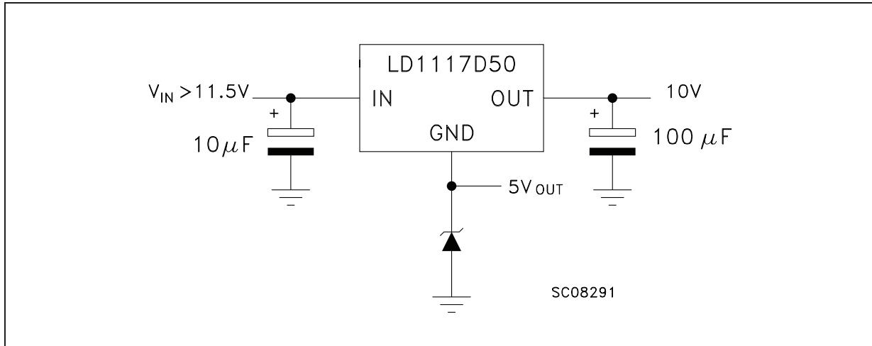
**Figure 9.** Battery backed-up regulated supply
