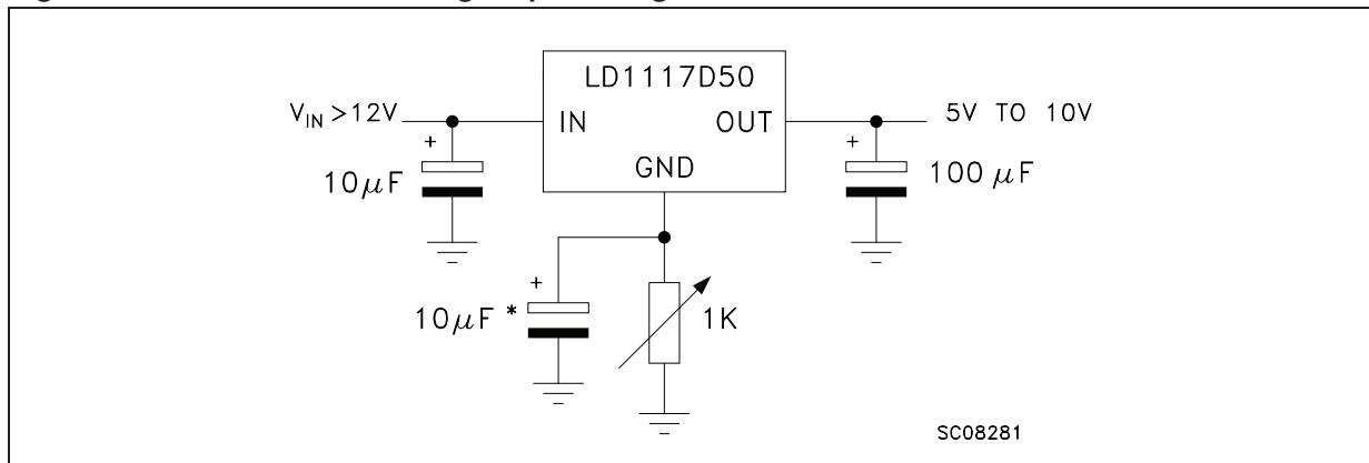
**Figure 8.** Voltage regulator with reference
