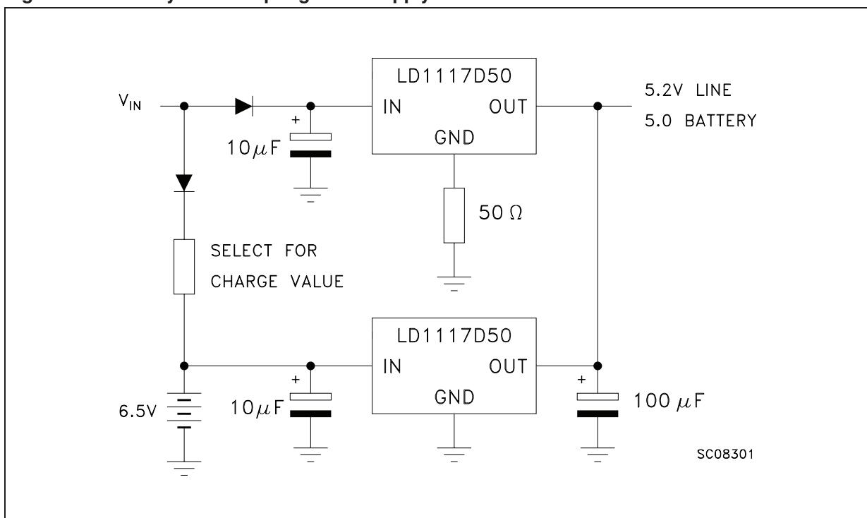
**Figure 10.** Post-regulated dual supply
