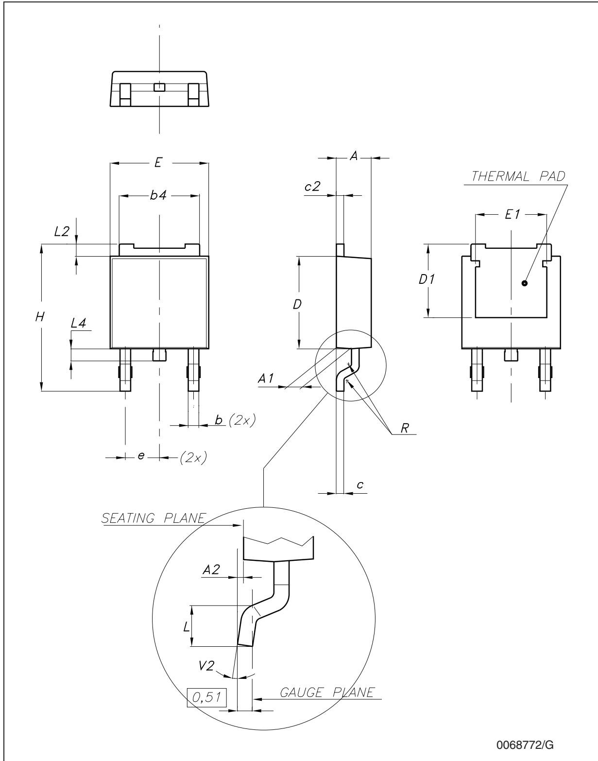
**Figure 19.** Drawing dimension DPAK (type IDS-subcon.)
