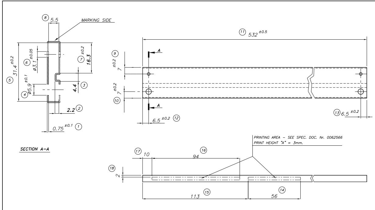
**Figure 16.** Drawing dimension tube for TO-220 Single Gauge (mm.)
