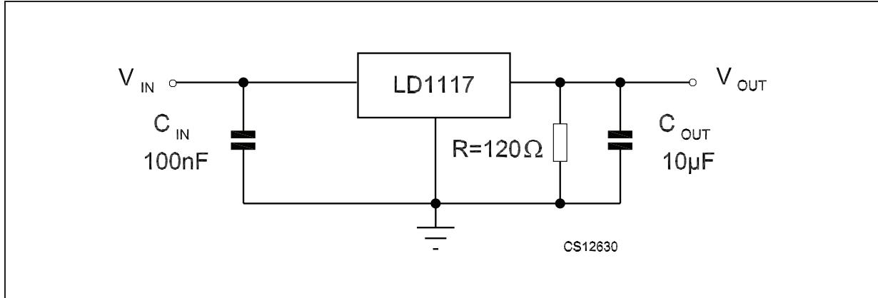
Figure 4. Application circuit (for other fixed output voltages)
