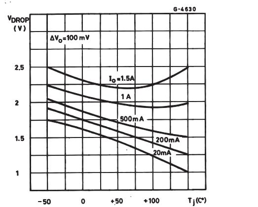
**Figure 5.** Reference voltage vs. junction
