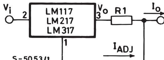
$$I_O = (V_{REF} / R_1) + I_{ADJ} = 1.25 \text{ V} / R_1$$
