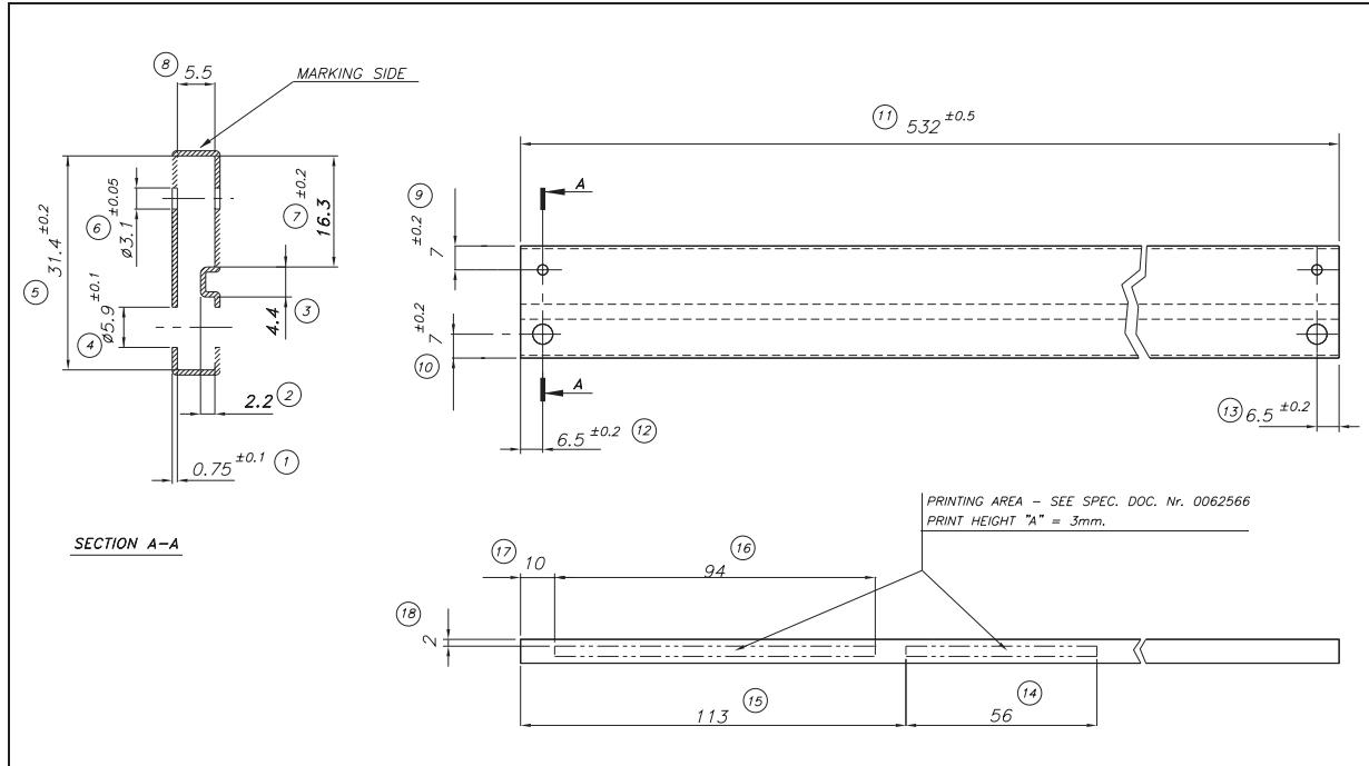
**Figure 17. Drawing dimension tube for TO-220 Single Gauge (mm.)**
