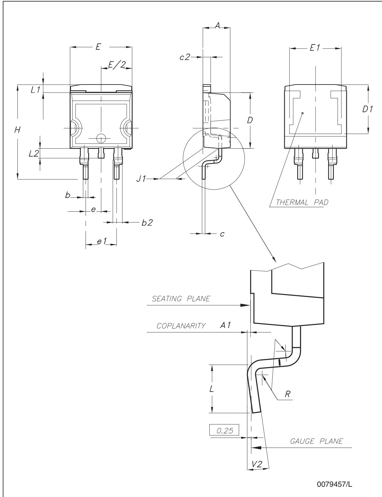
**Figure 19.** Drawing dimension D<sup>2</sup>PAK (type WOOSEOK-SUBCON.)
