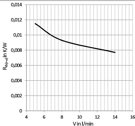
Fig. 9: Thermal resistance  $R_{\text{th}}(r-a)$  versus flow rate  $V$
