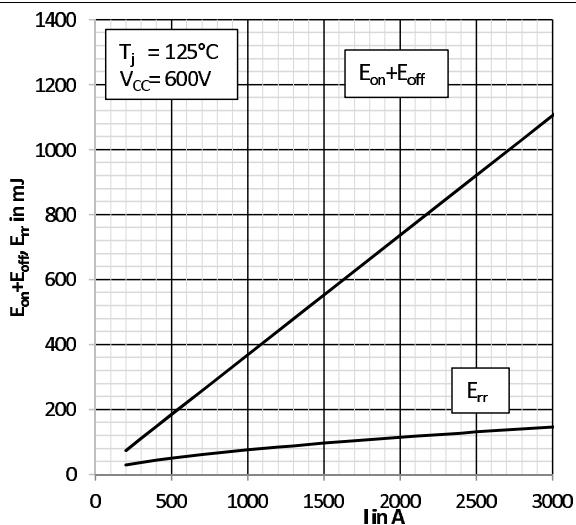
Fig. 3: Typical energy losses  $E = f(I_c, V_{cc})$
