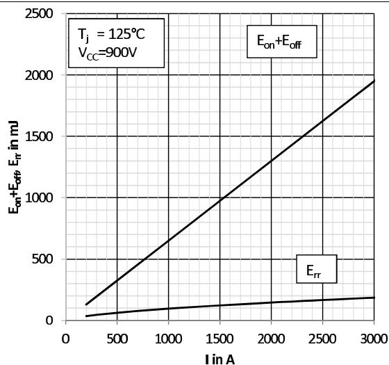
Fig. 4: Typical energy losses  $E = f(I_c, V_{cc})$
