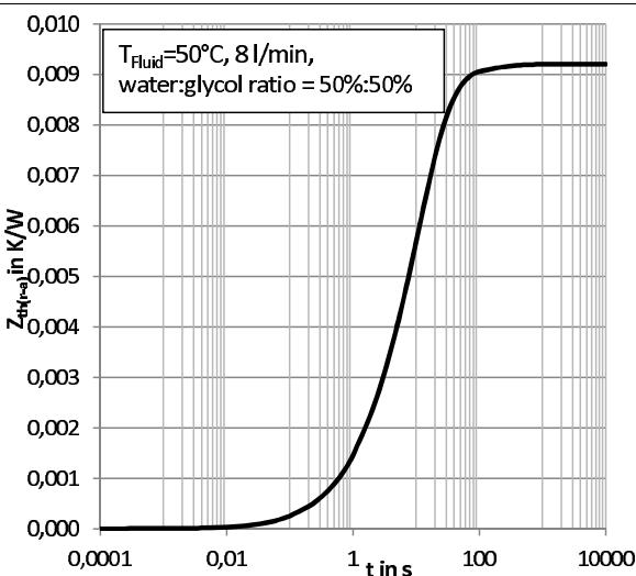
Fig. 7: Transient thermal impedance  $Z_{\text{th}}(r-a)$
