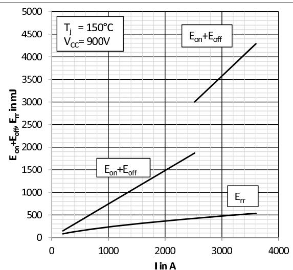
Fig. 3: Typical switching energy  $E = f(I_c)$
