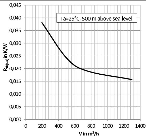
Fig. 9: Thermal resistance  $R_{th}(s-a)$  versus flow rate  $V$
