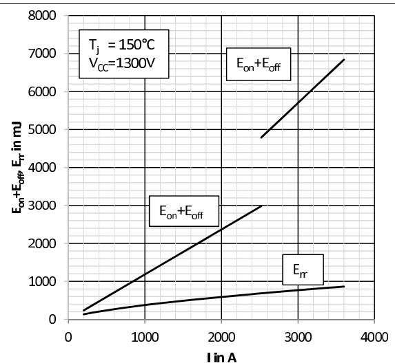
Fig. 4: Typical switching energy  $E = f(I_c)$
