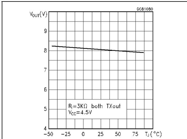
**Figure 8. Low level output voltage swing vs temperature**
