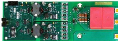
The MSCSICSP3/REF2 is a half bridge driver compatible with SP3F standard package modules.
