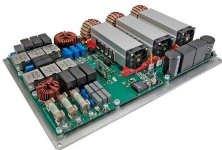
The MSCSICPFC/REF5 is a Vienna 3-Phase PFC reference design for Hybrid Electric Vehicle/Electric Vehicle (HEV/ EV) charger and high-power switch mode power supply applications.
