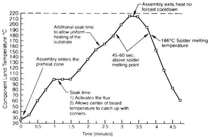
Recommended Ramp Rate Less than 2°C/sec.
