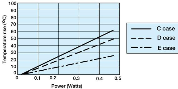
Several capacitors were tested and the combined results are shown above. All these capacitors were measured on FR4 board, with no other heatsinking. The ripple was supplied at various frequencies from 1KHz to 1MHz.
