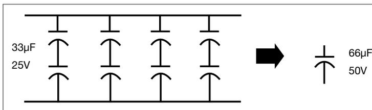
In order to ensure reliable operation, the capacitors should be connected as shown below to allow current sharing of the ac noise and ripple signals. This prevents any one capacitor heating more than its neighbors and thus being the weak link in the chain.
