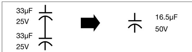
effective capacitance will be halved, so for greater than  $60\mu\text{F}$ , four such series combinations are required, as shown.
