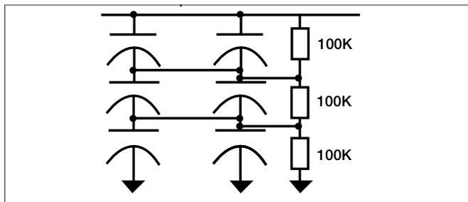
The two resistors are used to ensure that the leakage currents of the capacitors does not affect the circuit reliability, by ensuring that all the capacitors have half the working voltage across them.
