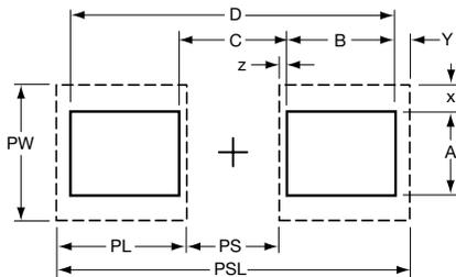
Dimensions PS (Pad Separation) and PW (Pad Width) are calculated using dimensions x and z. Dimension y may vary, depending on whether reflow or wave soldering is to be performed.
