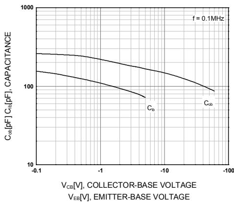
**Figure 3. Output and Input Capacitance
