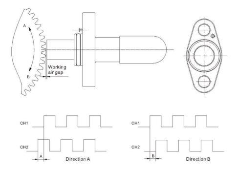
Fig.1 Rotation Direction Definition and Phase Relationship
